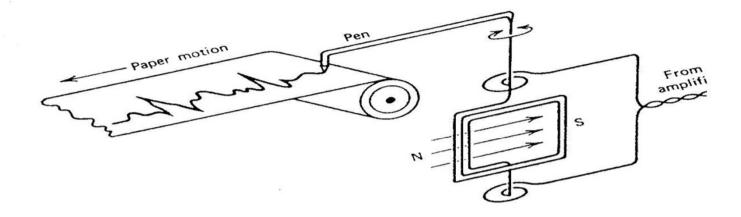
After amplification, the ECG signal must be displayed. When a routine diagnostic ECG is taken, a permanent record is required for analysis and a pen recorder is usually used (Fig.3). In a pen recorder, the amplifier output passes through a coil of wire suspended in a magnetic field. In the same way that a galvanometer twists when current passes through it, the pen twists to write on a moving strip of paper.
